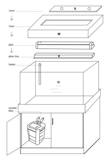
Place aquarium **U** on top of cupboard by lifting it on from the back and sliding it forward.
