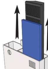
Remove sponge and carbon cartridge. If the carbon cartridge is due for replacement, discard it.
