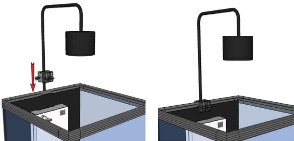
Fit the light mounting bracket to the back panel of the aquarium
