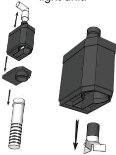
Remove elbow, intake strainer, impeller cover and then the impeller.
