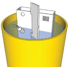
Rinse all other components of the filter to remove any debris or algae.
