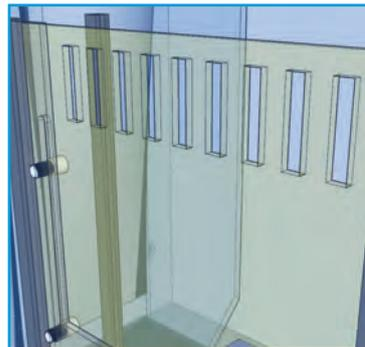
Check the grille on the movable baffle for blockages. If only part of the grille allows water through, it can become noisy.
