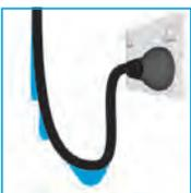
Arrange a drip loop for each cable to stop water entering the power socket. If the plug or the socket does get wet, disconnect the fuse or circuit breaker before unplugging the power plug.
