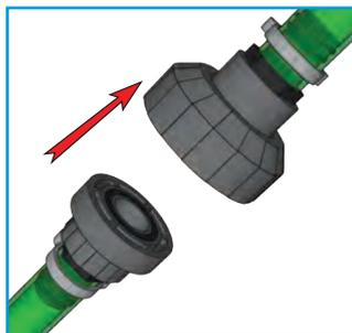
To remove the return pump for maintenance, first disconnect the quick coupling as shown.
