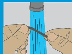
Put a small amount of lubricant\* on and smear it over the o-ring so that it is covered by a thin film.
