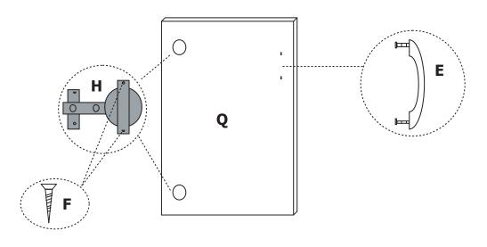
Step 6: Attach door Q to cabinet using screws F into the predrilled holes. Use parts F x 4.
