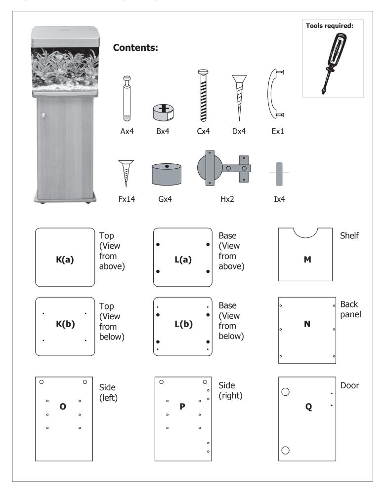
Step 1: Install the locking nuts & screws. Attach sides to top K(b) and Base L(b). Use panels K(b), L(b), O, P. Use parts A  $\times$  4, B  $\times$  4, C  $\times$  4
