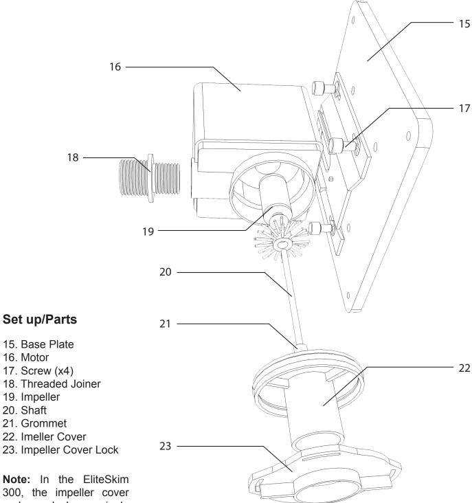
Note: In the EliteSkim 300, the impeller cover and cover lock are a single piece.
