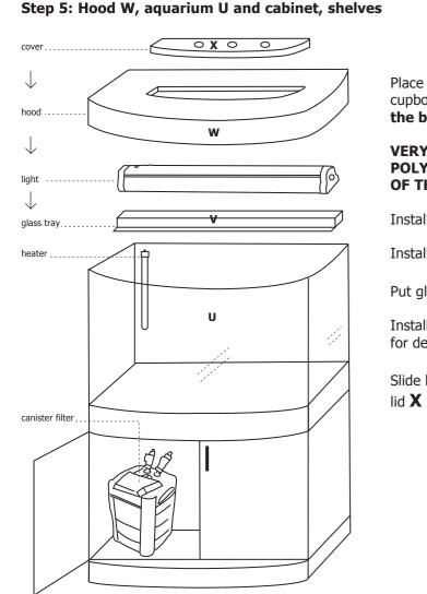
Place aquarium **U** on top of cupboard by lifting it on from the back and sliding it forward.
