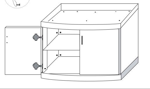
Lower side and back panels onto the base and secure screws B
