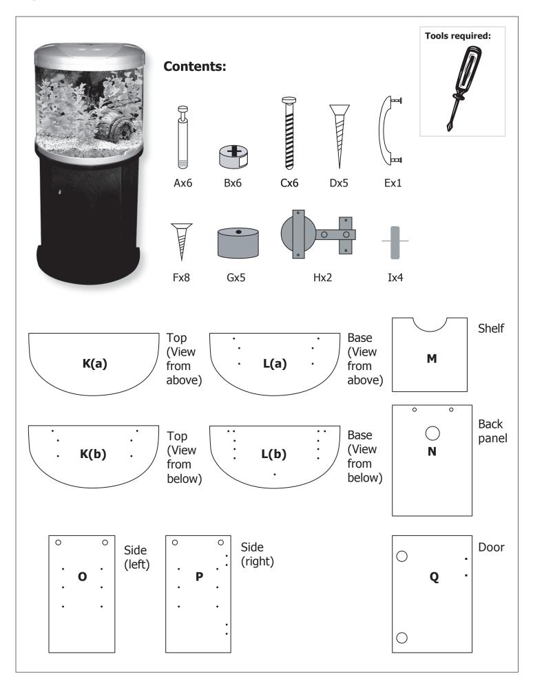
Step 1: Use panels K(b), N, O, P. Use parts A x 6, B x 6. Install the screws A x 6 to panel K(b) and locking nuts B x 6 to panels N, O, P, then attach the back panel N to K (b) and lock.
