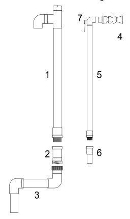
drain pipe so they can be connected using the barrel union.
