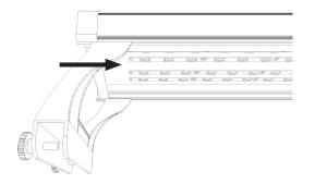
2. Mount the light unit on the side of the aquarium. Adjust the mounting brackets to the appropriate locations so that the brackets sit on the edges of the aquarium. Secure the light unit using the screws on the outside of the mounting brackets. Ensure the light unit is centred over the aquarium.
